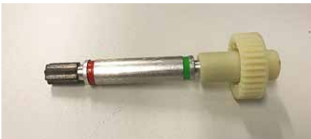
Figure 4: Example of a key quality control test of the star shaped axis of the plastic part. The plastic parts produced using the laser textured inserts fulfilled this quality criterion, even after reducing the cooling time by five seconds.
