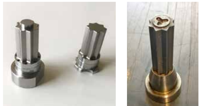
Figure 1 Left: Original star-shaped inserts of the production mould. Right: Test insert for studying the effect of surface treatments on the demoulding properties. All parts are made in stainless steel (1.2379).
